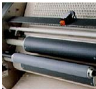
The sheeting unit consists of 2 plastic cylinders (food safe), fixed on tight ball bearings
