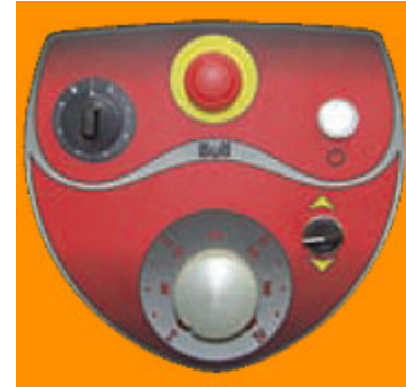
Bull Mixer Control Panel with Speed Variator
